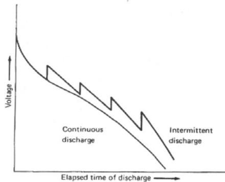
**FIGURE 3.12** Effect of intermittent discharge on battery capacity.
