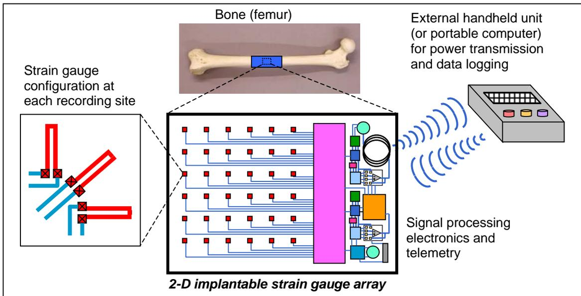
Figure 1. Diagram of an implantable, wireless, strain-sensitive membrane array. The gauge configuration at each recording site allows the complete stress state to be measured.
