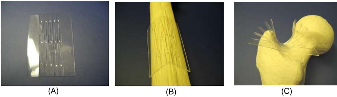
Figure 2. (A) Slotted prototype membrane, as fabricated (5cm × 7cm, 1mm thick). (B) Membrane along bony ridge on posterior aspect of femur. (C) Membrane shows good conformation to bone surface.
