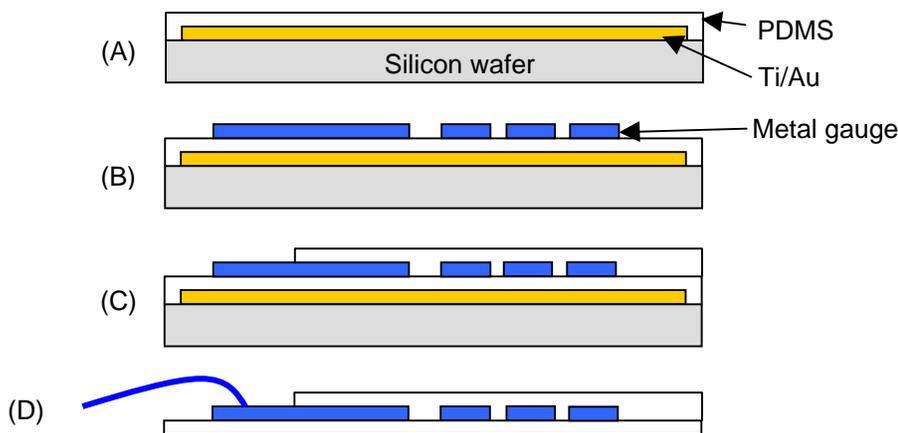
Figure 3. Device cross-section shown at each step. (A) Evaporate thin layer of Ti/Au to facilitate later removal of PDMS from the wafer. Spin on first layer of PDMS. (B) Evaporate and pattern metal gauge. (C) Spin on second layer of PDMS. Use stencil mask to protect bonding pads on electrodes). (D) Bond wires to electrode pads, Cut and peel device off the substrate.
