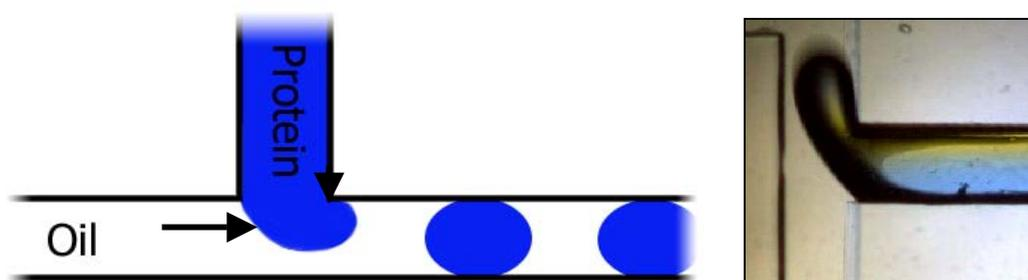
Figure 2. Protein droplet formation in oil. Droplet formation is highly controllable and very rapid. Droplets of sub nanoliter volumes can be generated at speeds of over 100 drops per second. Image on the right shows preliminary data from a microfluidic chip using this technology.
