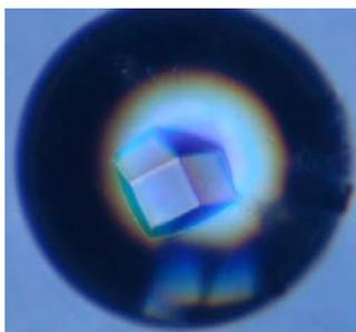
Figure 1: Image of a protein crystal grown in two nanoliters of solution. Typical crystals are grown in microliters.
