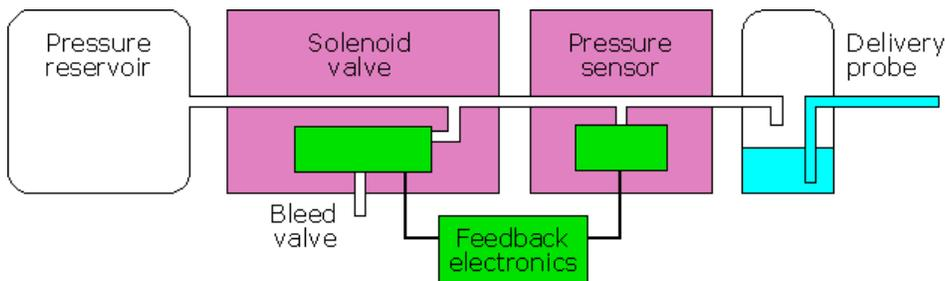
Figure 4: Diagram of operation for a computer controlled pressure delivery system.
