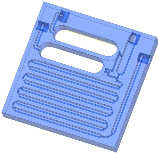
Figure 3: Design of microfluidic chip with serpentine section for storing nanodrops.
