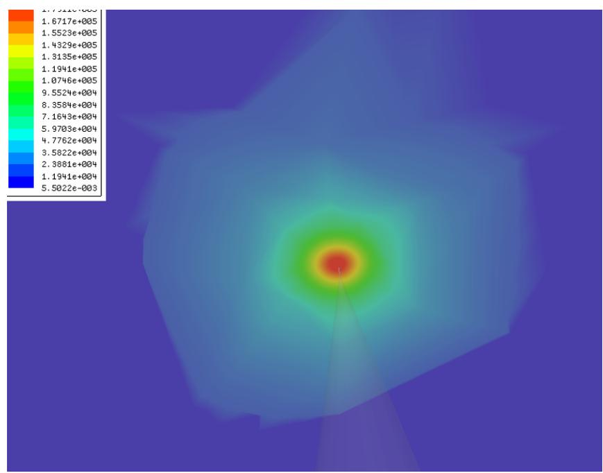
Fig. 8. Localization of electric field with tip-sample distance  $10^{-3}$  in.
