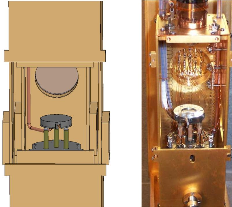
**Fig. 3.** HFSS model (left) (shield doors hidden) and actual STM (right) (shield doors removed).
