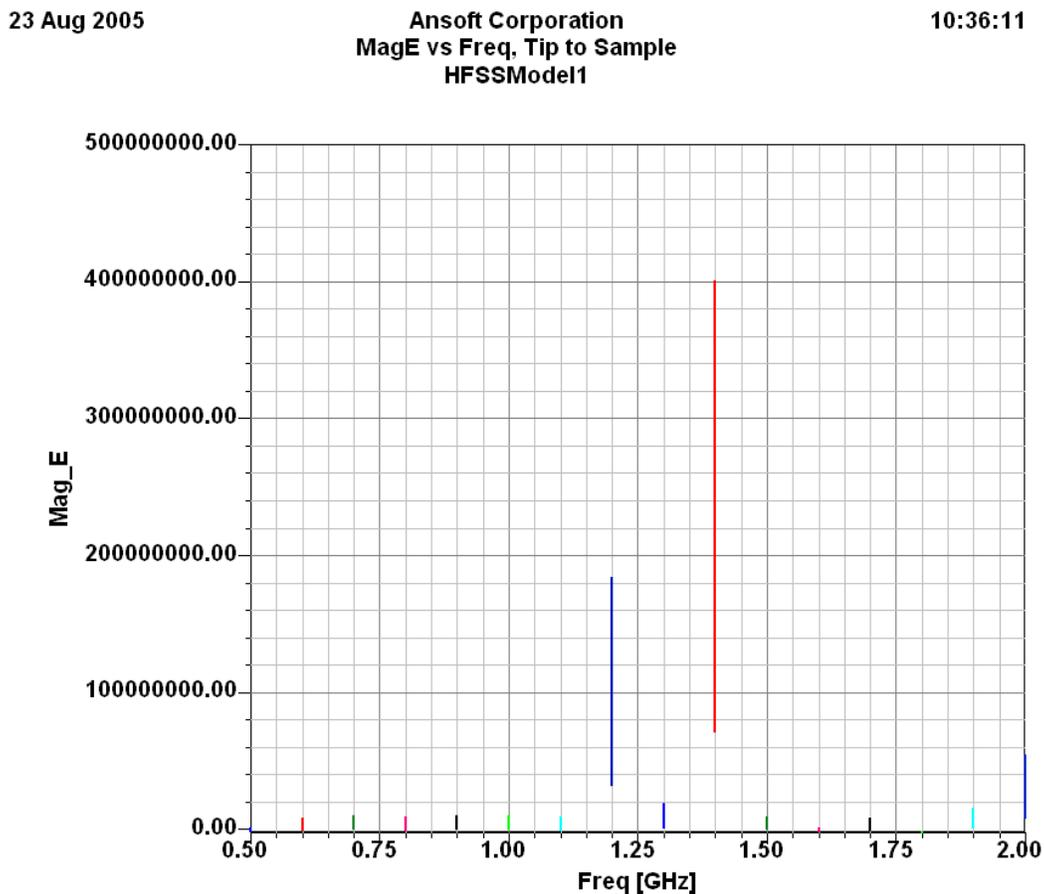
**Fig. 5.** Magnitude of electric field from tip to sample versus frequency with tip-sample distance  $10^{-6}$  in.
