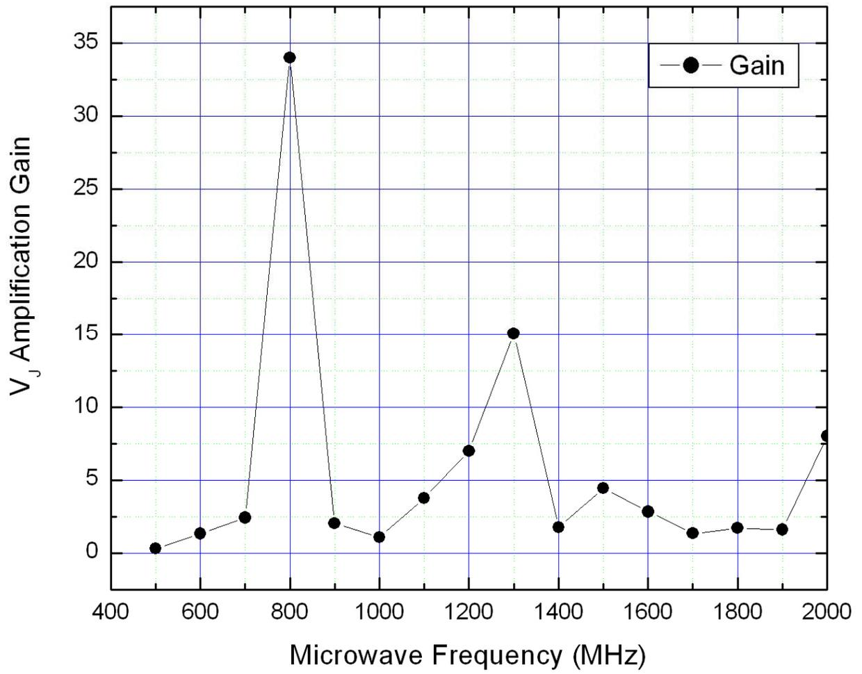
**Fig. 2.** Experimental results showing resonance at 800MHz, 1.2GHz, 1.3GHz, and 2.0GHz.
