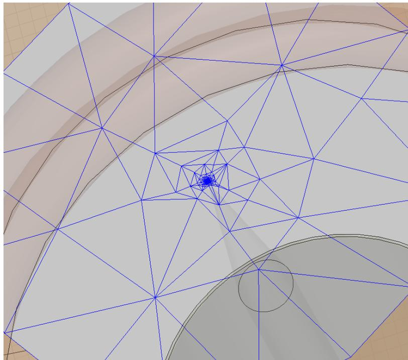
**Fig. 4.** Plot of mesh on bottom of sample. The outer circle (gray) has radius 0.09 in, while the small blue center, blue due to the extremely refined mesh, is a circle with radius 0.001 in.
