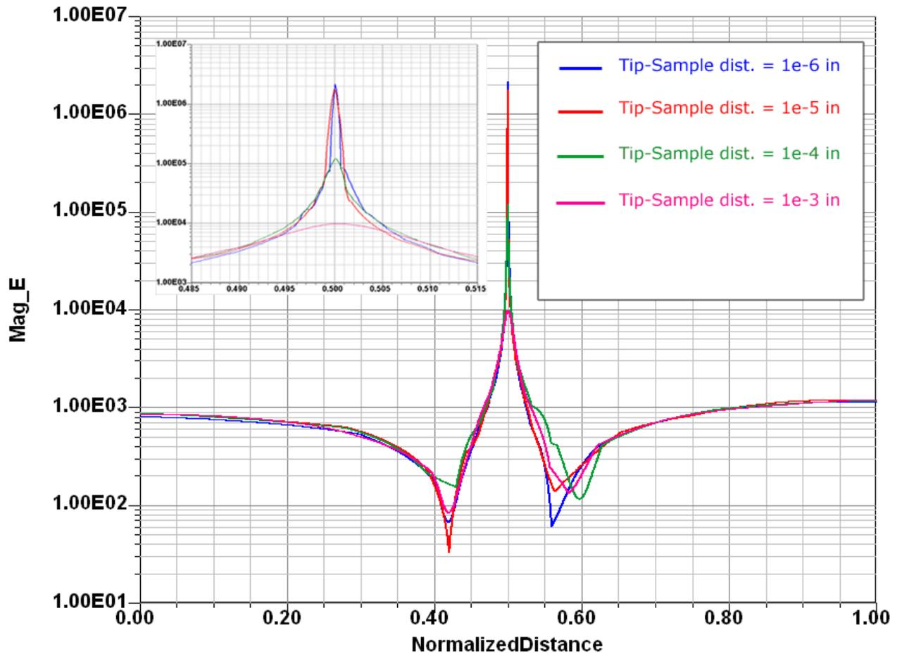
Fig. 6. Magnitude of electric field versus distance across sample. Left inset shows details of E field localization.
