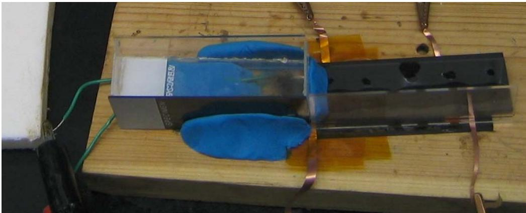
**Figure 6: Smoke generation chamber attached to millimeter scale visualization channel and sealed with Play-Doh**
