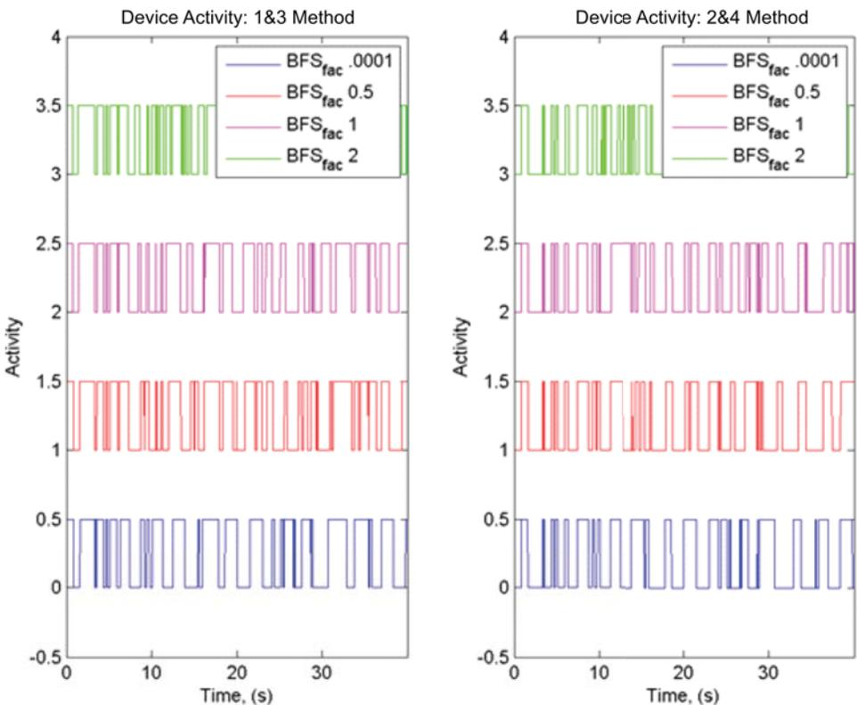
Figure 6 Activation graph for a Pulse-Like ground motion; values at 0.5 intervals represent an active device, while integer intervals represent a dormant device. As a check, the activity for the device under the 1&3 and 2&4 control algorithms should be opposite at similar temporal points during the seismic event.
