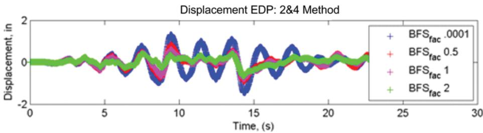
Figure 5 Comparison plot of total Displacement EDP response from the brace-frame system under varying BFS factors. Note that a BFS factor of .0001 is essentially equivalent to a system without the energy dissipating device, operating only under an assumed natural structural damping of 5%.
