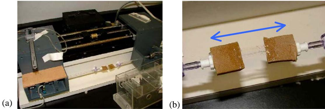
Fig. 7: a) Photo of tensile tester. b) Close-up of device under test. Device is subject to tensile forces until breaking. Direction of applied force shown (blue arrow). Device is glued on either end to rigid foam using silicone sealant.
