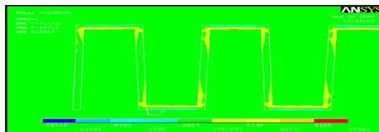
Fig 4: Simulated contour plots of the reference strain gauge by ANSYS with a tensile stress of 10 Pa applied along  $x$ -axis. The color scale shows the stress value range from  $-14719$  Pa (dark blue) to  $12083$  Pa (red). The green background indicated the value of stress acting on the PDMS to be  $-2807$  Pa. High stress areas are in the corners of the gauge, as expected.
