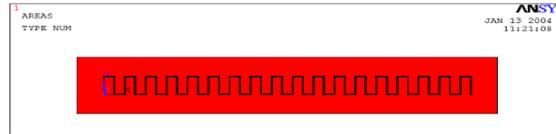
Fig 2. Undeformed 18 turn gauge embedded in PDMS. The black regions represented the metal while the red represents the surrounding PDMS membrane.
