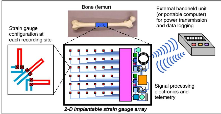
Fig 1. Diagram of an implantable, wireless, strain-sensitive membrane array. The gauge configuration at each recording site allows the complete stress state to be measured.
