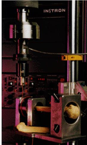
Fig 8. MTS servo hydraulic tester. The tester will allow tension, compression and torsion tests [8].
