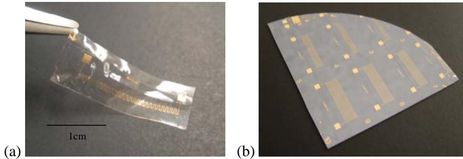
Fig. 6: a) Fabricated gauge with a thin film of gold sandwiched between two layers of 50 $\mu$ m thick PDMS. b) Array of gauges on one quarter of a silicon wafer, prior to wire bonding and peeling off the substrate.
