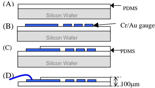
Fig 5. A) PDMS is spun on a silicon wafer. B) Metal is patterned on PDMS using photolithography C) A second layer of PDMS is spun on, which encases the metal gauge. D) Device is peeled off silicon wafer and is tested.
