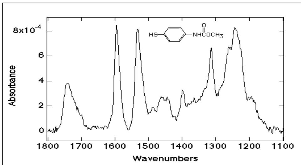
**Figure (5):** PM-FTIRRAS spectrum of an alkanethiol monolayer on a vapor-deposited gold film after normalization of data<sup>(8)</sup>.
