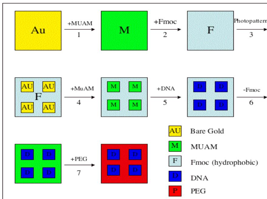
**Figure (2):** Fabrication Scheme for the construction of multi-element DNA arrays. Note that this is a simplified scheme, and the one I intend to use for experimentation will consist of 16 probes attached to one surface. A clean gold surface is reacted with MUAM, and subsequently reacted with Fmoc-NHS to
