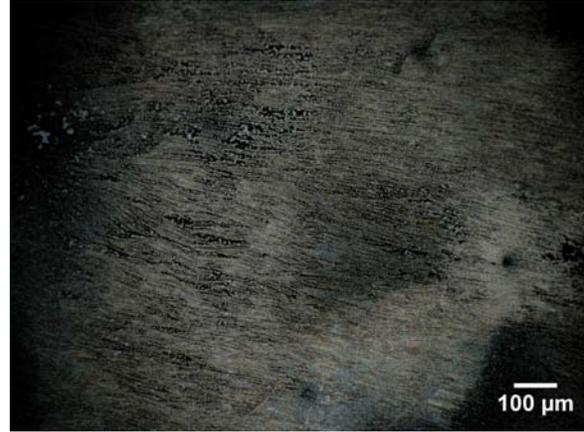
**Figure 9. NiTi wires created by a CV with the cycle 0V → -2.5V → 2.5V → 0V at 50mV/sec.**
