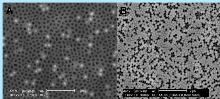
Fig.2: A. DC electrodeposition; B. PED. Notice how filling factor is much improved in B.
