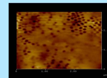
Fig. 6: Zn starting to become ZnO on the surface of the pores.
