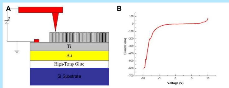
Fig.4: Schematic of the AFM measurement. The *I-V* curve in B shows a Schottky contact between the probe and the nanowire.
