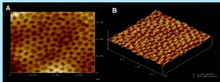
Fig.3: A. AFM picture of the AAO membrane filled with Zn nanowires. B. 3-D view of the same image. Density is approximately 70%-80%.
