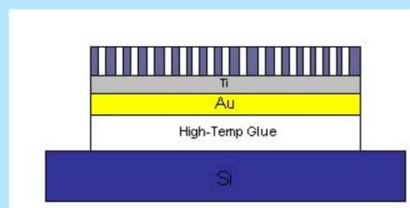
Fig.1: Schematic of the chip before PED
