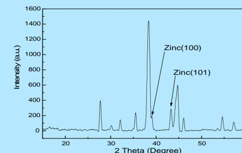
Fig. 5: XRD data confirming the presence of Zn in the chip.
