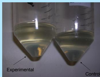
Figure 6. A photo showing visual contrast between oil passed through control and experimental setups.
