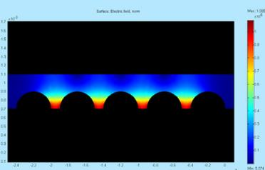
Figure 1. Simulation of the electric field distribution between semicircular electrodes.
