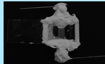
Figure 3. Photo of one of the first prototypes. (6 steel electrodes sandwiched between two microslides sealed with PDMS and Silicone II.)
