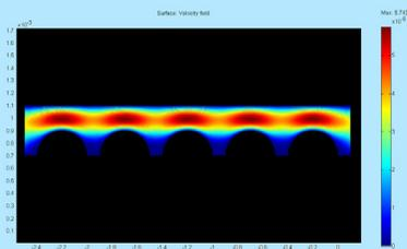
Figure 2. Simulation of the velocity field distribution for semicircular electrodes within a fluidic channel.
